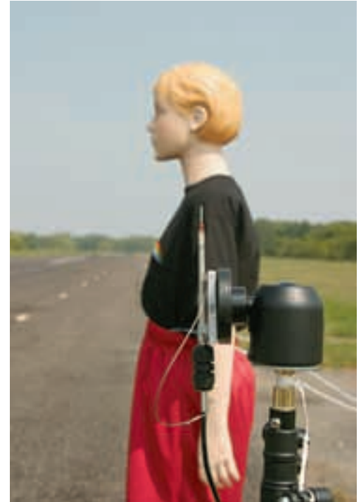
The air speed sensor measures the magnitude of the air turbulence produced by the passing truck.
