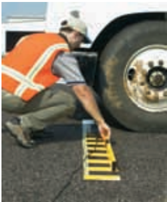
The tire tape switch records the position and speed of the passing vehicle.
