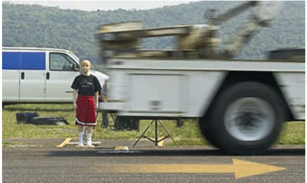
In all tests conducted, the mannequin never moved when the truck drove by. Obviously, the child's injuries were not caused by being sucked under the truck's rear tires.
