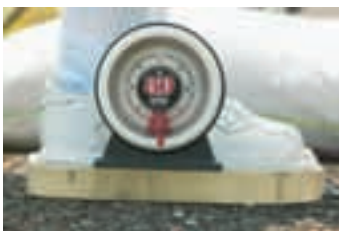
The scale ensures that the mannequin's static balance is the same as the child's.
