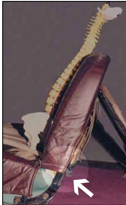
When weight equivalent to the truck driver's was applied to the seat, an analysis with an anatomically correct spine model clearly showed that the location of the bent seat frame corresponded exactly to the location of the spinal disc that was injured.
